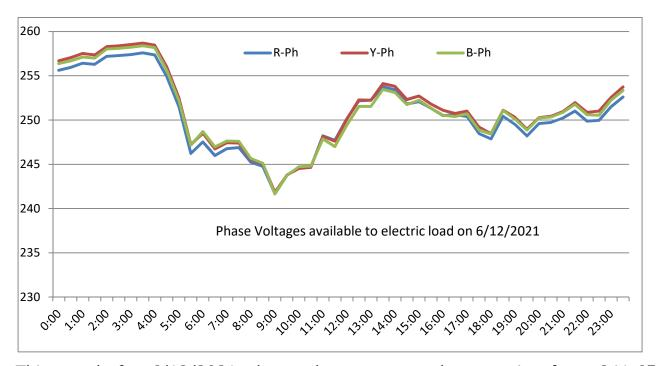
This graph for 6/12/2021 shows that system voltage varies from 241.65V to 258.69 V against 433V and hence all the electric load connected rated generally for 230V consume more power proportionate to square of the voltage and it is recommended to change the voltage at Distribution Transformer off load tap changer such that load do not get voltage more than its rated 230V.
