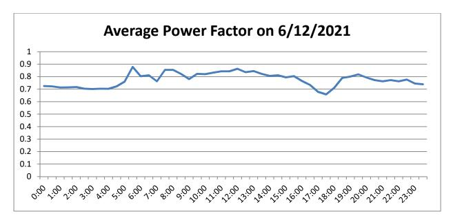
The power factor has been recorded as min as 0.030 (on 19/12/2021, 10:30AM) with 135A load and as maximum as 1.000 with average power factor 0.747. It is necessary to maintain average power factor (both lagging & leading) with minimum value of 0.900, failing which penalty is imposed in every energy bill and sometimes becomes liability on the administration for paying penalty amount.
