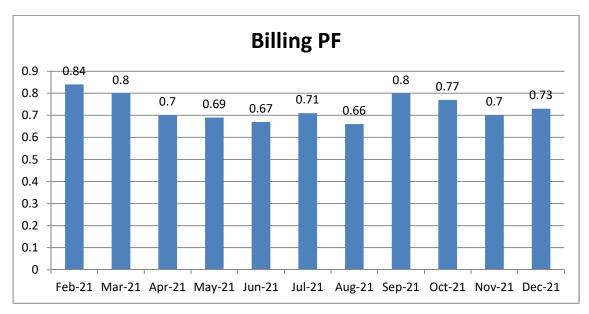
The Poor Power factor from Feb-21 to Dec-21 have resulted into payment of cost of 13442 kWh as penalty (>Rs. 1.0 lacs), and therefore, it is recommended to install APFC panel to maintain power factor >0.90.
